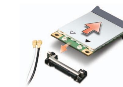
Mobile Broadband card slot locations vary by computer model. See your computer User's Guide for location and access instructions. After accessing the card slot, move the antenna cables out of the way and insert the Mobile Broadband card as shown.
