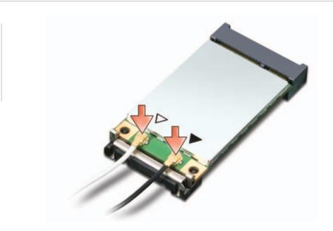
Connect the appropriate antenna cables to the Mobile Broadband card you are installing. To do so, connect the white with gray striped cable to the connector on the card marked by a white triangle. Connect the black with gray striped cable to the connector on the card marked by a black triangle.
